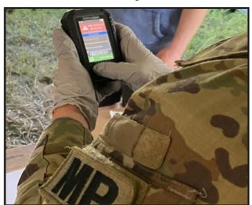
Explosive residue tests for the exercise were conducted by 527<sup>th</sup> Military Police Company Soldiers using the SEEKERe, an automated colorimetric handheld device. (U.S. Army photo)
