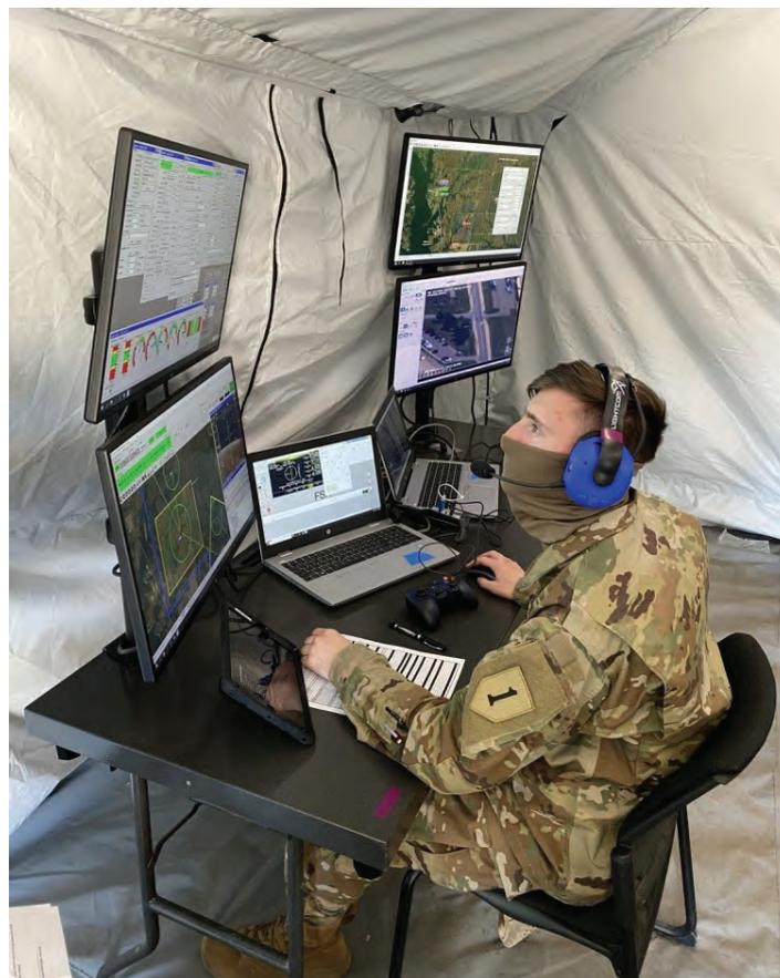
A U.S. Army Soldier assigned to 1<sup>st</sup> Engineer Battalion, 1<sup>st</sup> Infantry Division, conducts flight operations through a laptop-based ground control station during the future tactical unmanned aircraft system capabilities assessment at Fort Riley, KS, April 8, 2020.
