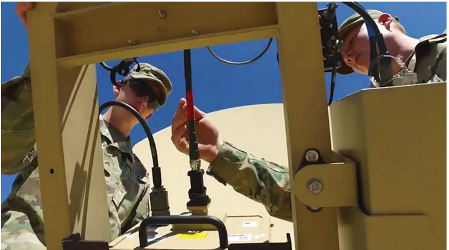
Military intelligence systems maintainers use testing and diagnostic equipment to troubleshoot and repair an intelligence system component.
