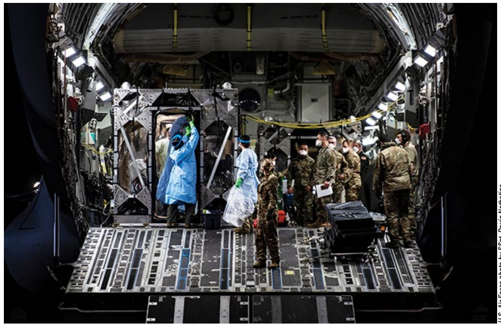
Airmen prepare to off-load COVID-19 patients during the first operational use of the Transport Isolation System (TIS) at Ramstein Air Base, Germany, April 10, 2020. The TIS is an infectious disease containment unit designed to minimize contamination risk to aircrew and medical attendants, while allowing in-flight medical care for patients afflicted by a disease—in this case, COVID-19.
